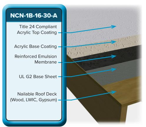
*WeatherWeld* NCN-1B-16-30-A is a completely seamless roof system designed for installation over nailable (plywood, poured gypsum or lightweight concrete) roof decks.
