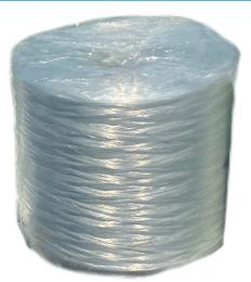
WWFG100 - Fiberglass Roving is continuous filament glass fiber consisting of approximately sixty strands held together loosely in rope form by a special sizing. Roving is designed for spray application using the WeatherWeld 3D Roof Printer to provide reinforcement for WeatherWeld asphalt emulsion coating.
