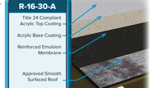
**WeatherWeld** R-16-30-A is a completely seamless roof system designed for installation over nearly all smooth and granule surfaced roof systems\*.
