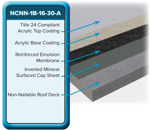
WeatherWeld NCNN-1B-16-30-A is a completely seamless roof system designed for installation over concrete roof
